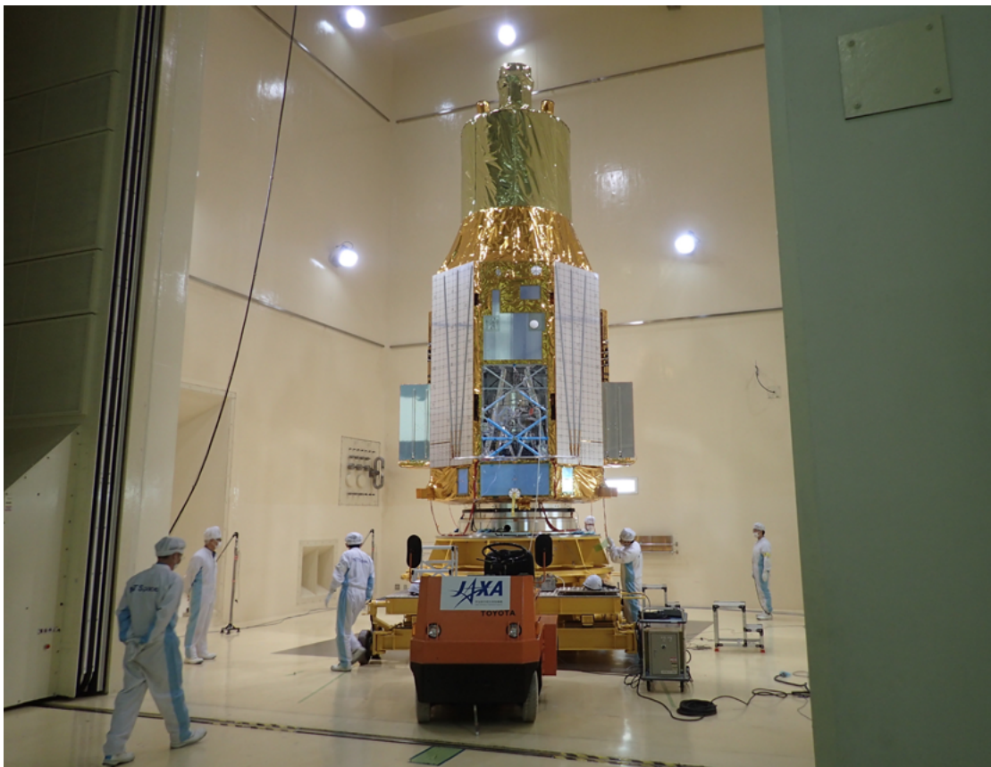
The fully assembled Astro-H spacecraft at JAXA's Tsukuba Space Center being prepared for acoustic vibration tests.
