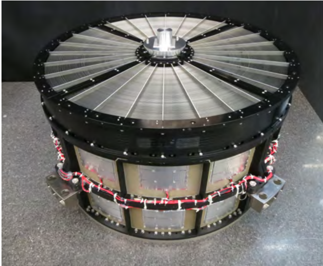
The X-ray mirrors produced for the Astro-H Soft X-Ray Imager (left) and SXS (right). The mirrors have 203 concentric reflectors, so contain 1624 individual, precisely aligned mirror segments. They are 45 cm in diameter and have a mass of 43 kg each.
