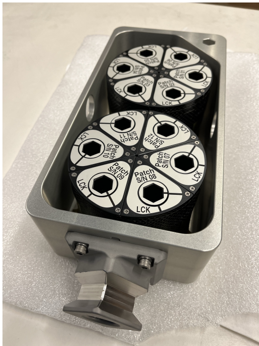
The NICER patch kit. Twelve triangular patches are shown installed within two flight-spare NICER sunshades, mounted in a rectangular aluminum caddy. This kit will fly to the International Space Station in August 2024, where crewmembers will carry it outside to install five of the patches at specified locations on NICER's X-ray Timing Instrument, covering holes created in May 2023 by orbital debris and restoring dark conditions within the XTI. The hexagonal hole at the center of each patch is designed to accommodate a tool already available to astronauts onboard ISS. Credit: K. Gendreau
