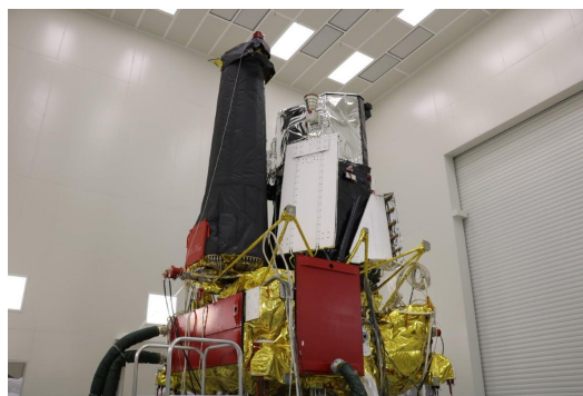
The eROSITA X-ray telescope integrated onto the SRG Navigator platform during the final assembly in September 2018 in the laboratory of NPOL Lavochkin, near Moscow. Credit: Lavochkin Association
