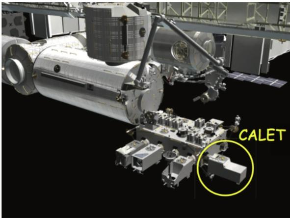
The Japanese Experiment Module-Exposed Facility on the ISS. CALET is attached at the #9 port as indicated. Credit: S. Torii and the CALET collaboration.
