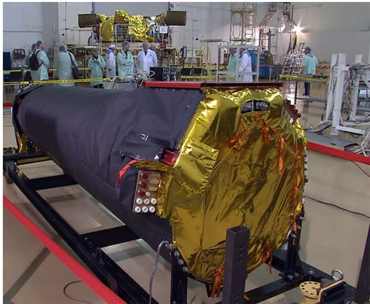
The ART-XC telescope in the NPOL assembly hall. Credit: MPE; IKI
