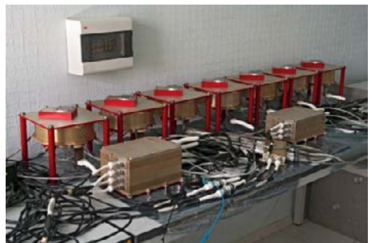
ART-XC X-Ray detectors system consisting of 7 detectors, 2 electronic boxes and one commutation box.
