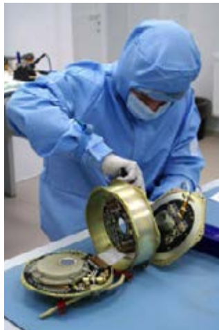
Final assembly of ART-XC X-ray detector unit.
