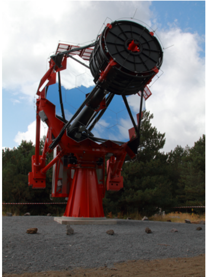
The 4m ASTRI telescope, inaugurated in Sicily on Sept 24th, 2014. It represents a prototype of the 70 Small Size Telescopes to be installed at the CTA southern site.
